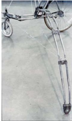
*Bike designed to move like an eagle riding air currents. Students observed that the arcs of the eagle's movements were similar to compass points. Bike turns when rider leans to one side activating the compass point at the tip of the wing. Wings made with bike forks, tension cables, and a roller blade wheel at the tip.*
